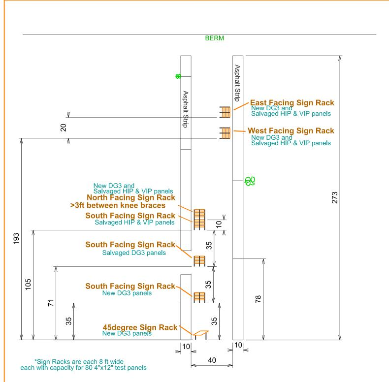
MNROAD SIGN TEST DECK LAYOUT (As-Built)
