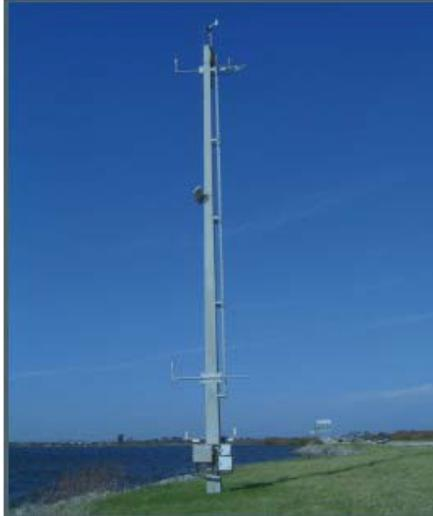
**Figure 3. ESS Above Ground Sensor**
